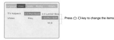
A. Press **ENTER** key to confirm B. Press **OSD/SETUP** key to return to stop mode [4:3 Letter Box]----In this mode a black band appears at the top and bottom. [4:3 PanScan]----In this mode the picture viewed appears to be cut from the left and right sides at a moment, but it actually scans the whole scene from left to right and vice-versa.
